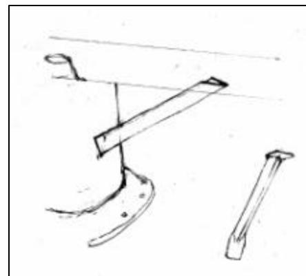
broader base which could facilitate welds further apart. This would require an extra step and the likelihood of a jig to perform the stamping.
