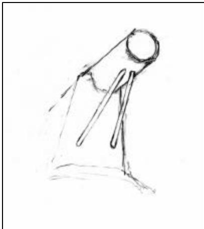
The next step in its evolution was the use of a dual support configuration, aimed at not only improving aesthetics, but distributing forces over a larger area across the base. Challenges presented by this iteration are the interface between the pedestal and base, and continued point loading issues. Again, the most obvious connection could be made with a TIG weld at the joint, performed cleanly, but could also be relatively easily done by
